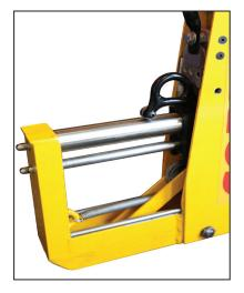
The guide rail or spring is damaged and is not pushing the staples forward. (return to distributor for service)
